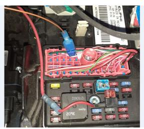
BCM 12V Brake Locations: C3/X3 A12 (Right Brake Lights) DK GRN A9 (Left Brake Lights) YEL
